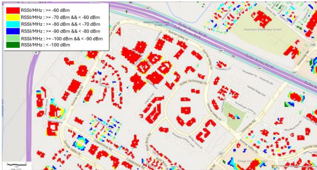
Figure 6: Predicted indoor signal strengths: Part 15. The red areas indicate the strongest signals while the green areas indicate the weakest.
